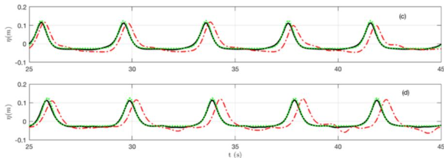
Free surface time history of a cnoidal wave. Dashed red line: IHFOAM (release 2014). Dotted green line: Theoretical solution. Black solid line: IHFOAM (OpenFOAM® release 17.06).
